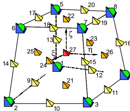
Figure 1. Finite element HC8/(9-27)
