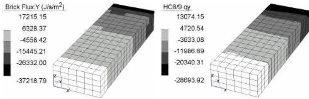
Figure 6: Heat flux  $q_y$  calculated by the primal (left) and present mixed approach (right)
