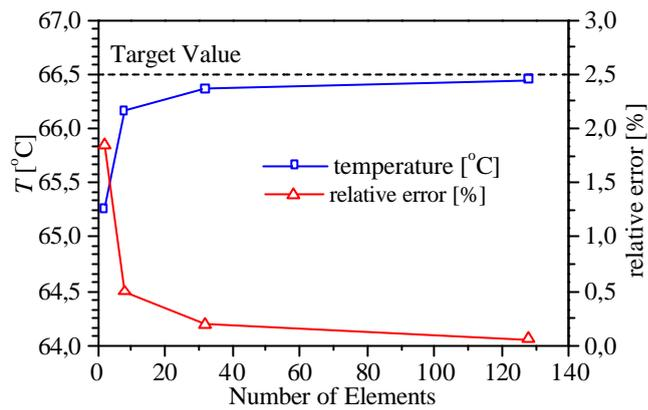
**Figure 8: Hollow cylinder: Temperature result at target point and relative errors**
