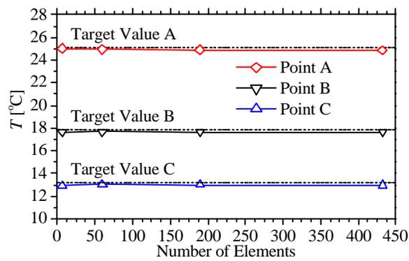
**Figure 10: Convergence of the temperature values on three radii of the sphere**
