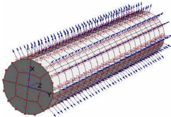
Figure 2: Cooling of the still rod model problem
