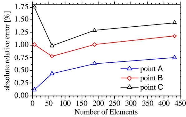
**Figure 11: Relative errors of calculated temperature values compared to the exact solutions**
