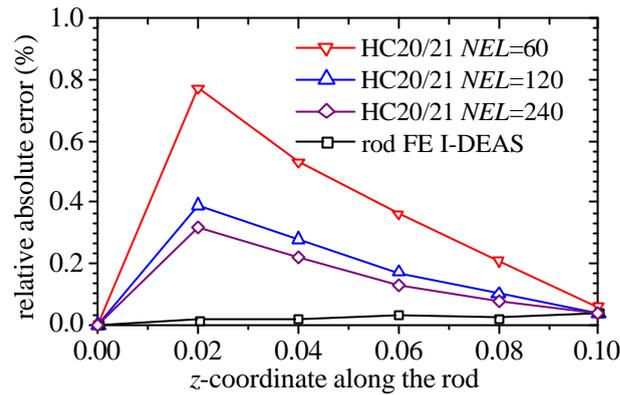
**Figure 3: Solid billet: The relative absolute error in accordance to 1-D theory**
