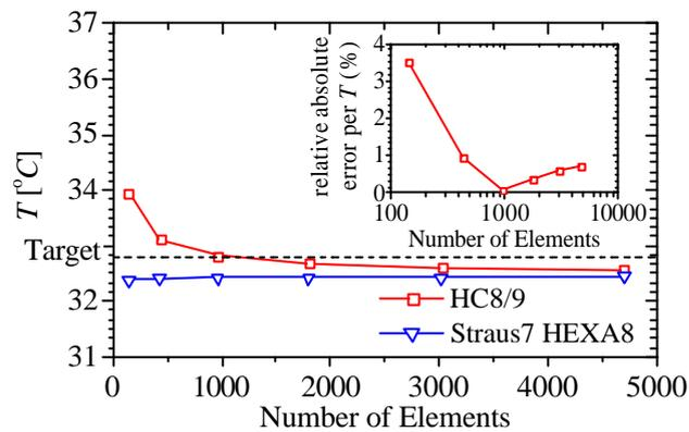
**Figure 5: Solid billet: The convergence of temperature at target point**
