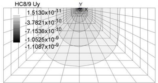
Fig. 9. Nanoindentation model: displacement field  $u_y$  after first increment of analysis of the whole model
