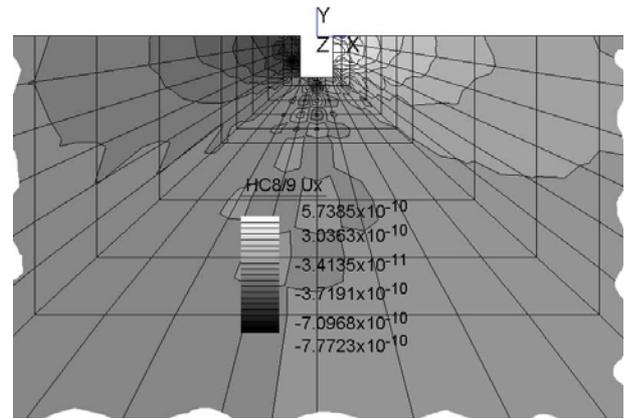
Fig. 10. Nanoindentation model: displacement field  $u_x$  after first increment of analysis in CM region near MD region after first increment of analysis
