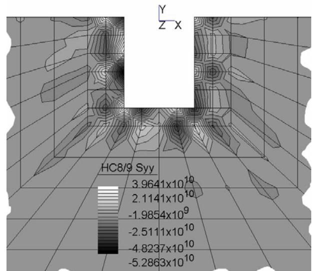
Fig. 11. Nanoindentation model: stress field in CM region near MD region after first increment of analysis
