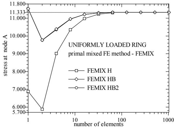
Figure 7: Uniformly loaded ring stress convergence at A
