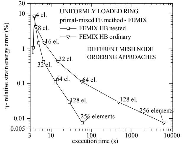
Figure 5: Efficiency as a function of node ordering
