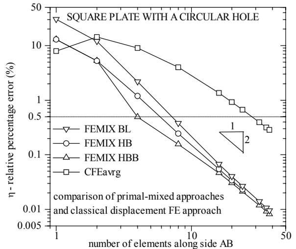
Figure 2: Percentage error versus number of elements
