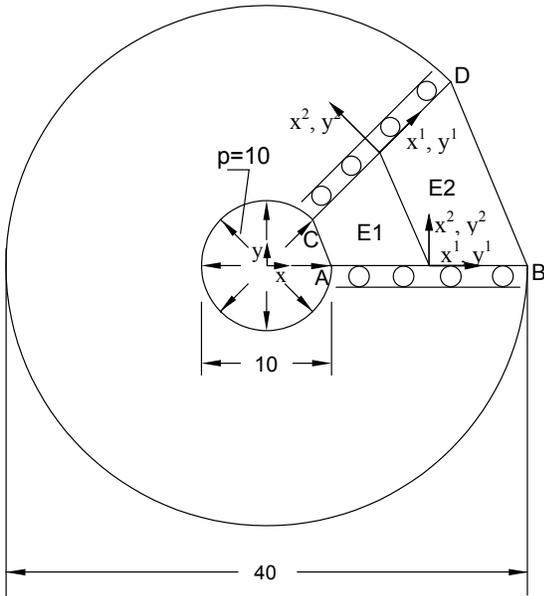
Figure 4: Uniformly loaded ring – model problem
