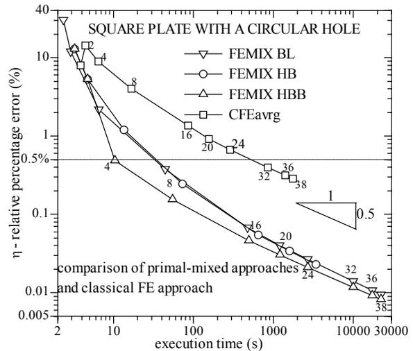
Figure 3: Percentage error versus execution time
